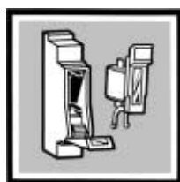
switching on without an inserted fuse is not possible
