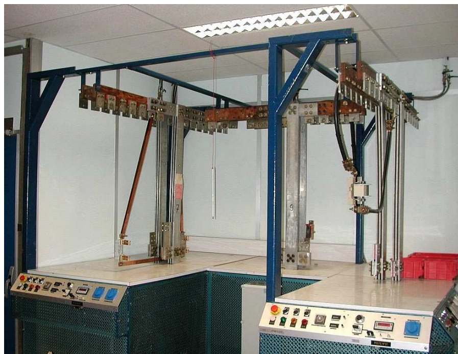
Temperature rise test station rated 4000 A
